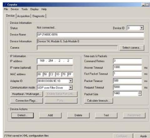
"Camera Link camera" is selected in "Select Camera" and press "Test". It will connect and "Status" changes to "Device connected". If you see an error message displaying "Cannot connect the Socket",
