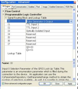
This PLC function is quite powerful and it is capable of performing many high level functions used in factory automation. Self triggering is one of the simplest applications.
