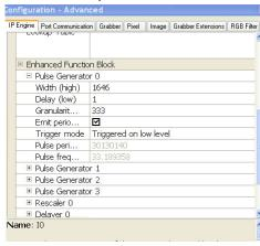
pulse form and unit (granularity) in ns. One unit is 30ns. Make sure that "Periodic" is marked to generate repetitive pulses. If you want single shot, you need a different triggering method. Since it is internal self triggering without any synchro-
