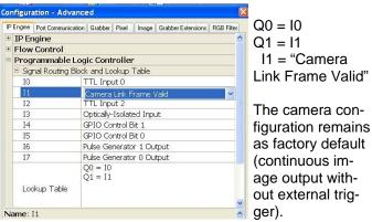
When GPIO pin #3 (green wire) is monitored, you will see pulses. Use negative going edge for the strobe triggering pint. The image will appear in the next FVAL-high period.
