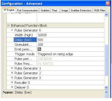
The delay is pulse state low and width is high. For pulse width control the camera looks low period as the exposure control and the total cycle as the trigger duration.
