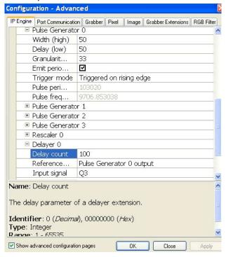
Also in Pulse Generator 0, set periodic and clock frequency. In this example, we set granularity to 33 to make 1 $\mu$ s pulse duration at minimum and Width and Delay for 50 each making 1 cycle of 100 counts (=100  $\mu$ s = 10KHz).
