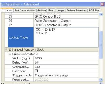
For this simple example, we keep the pulse generator with periodic (continuous) mode. Mark "Emit periodic "
