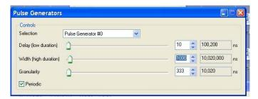
In this application, the frame rate is controlled with three parameters. For the simplest use, you can choose Width variation as the variables. Since the Granularity is set at 10µs as unit, any multiple of Width dictates the frame rate. In the sample, 1000 represent 10ms of frame rate = 100 fps. If 25 fps is required, set the Width to 4000 (=40ms = 25fps).
