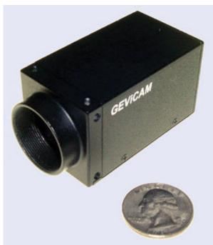
One of the smallest GigE cameras on the market, the GEViCAM VGA-based camera measures 34 × 34 × 60 mm. Future versions will incorporate a neural-network-based image processor in the package.
